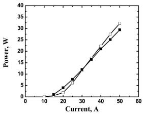
Fig. 3. cw output power of a free-running (empty square) and a volume Bragg (filled square) LDBs versus driving current.
