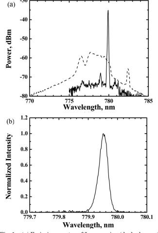
Fig. 1. (a) Emission spectra of free-running (dashed curve) and volume Bragg (solid curve) diode lasers in semi-log scale. (b) Emission spectrum of a VOBLA in linear scale.
